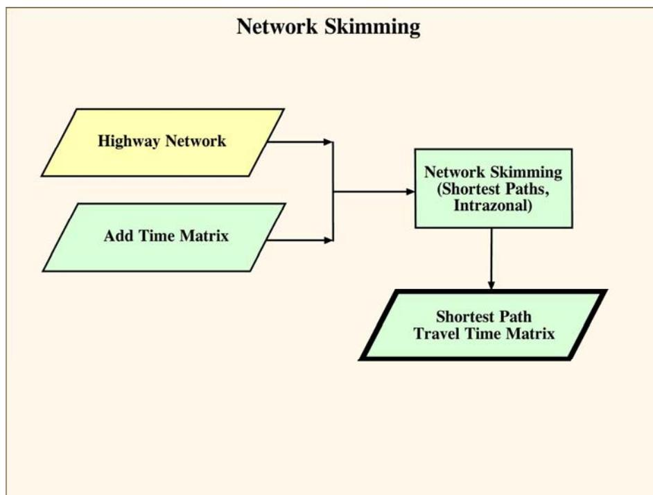
The roadway network (.NET) file created in the “Network Creation” process serves as one of the inputs in this process.
