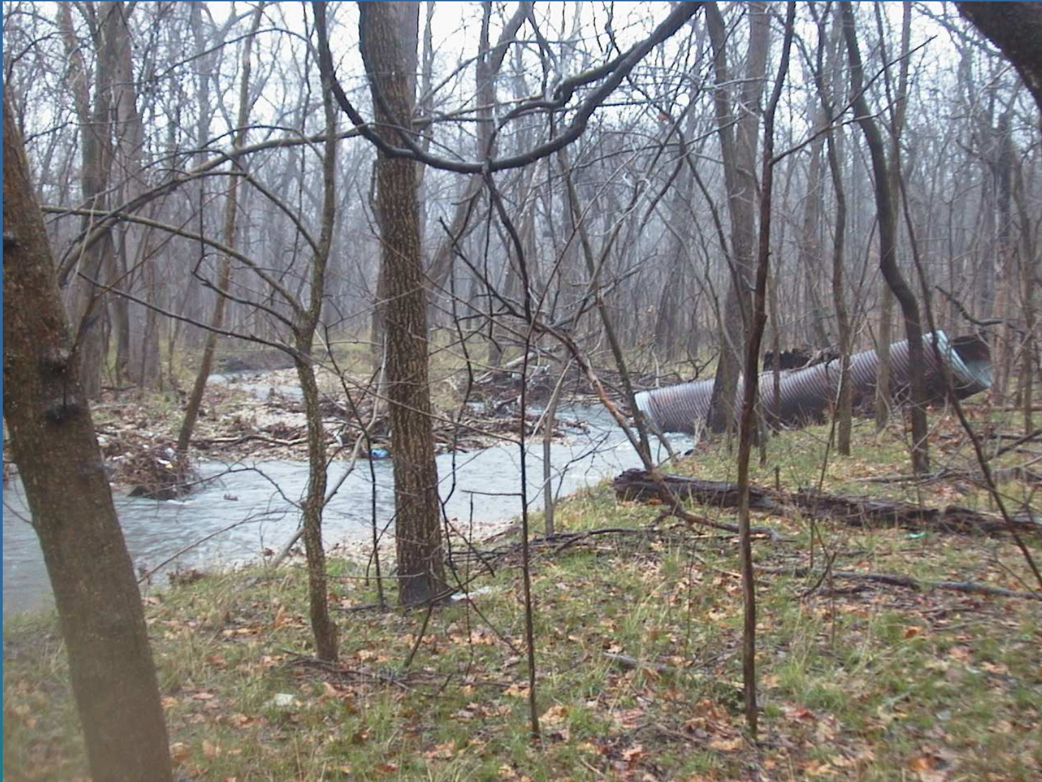
Failed pipe from WalMart site downstream!
